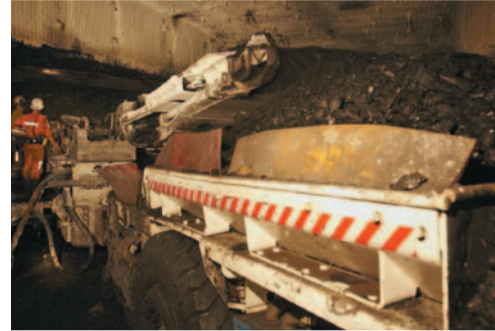
Shuttle car loading coal from the continuous miner.
