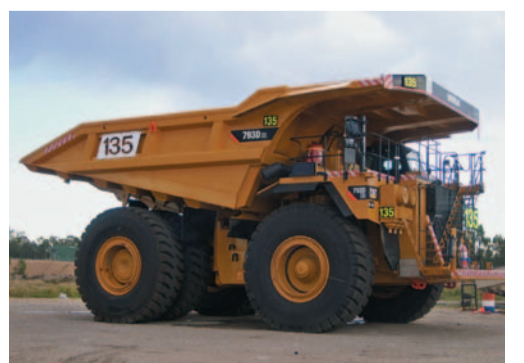
One of two new noise attenuated Caterpillar 793 commissioned in December 2009.
