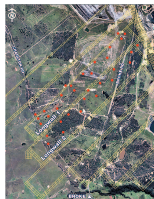
Goaf drainage wells.
