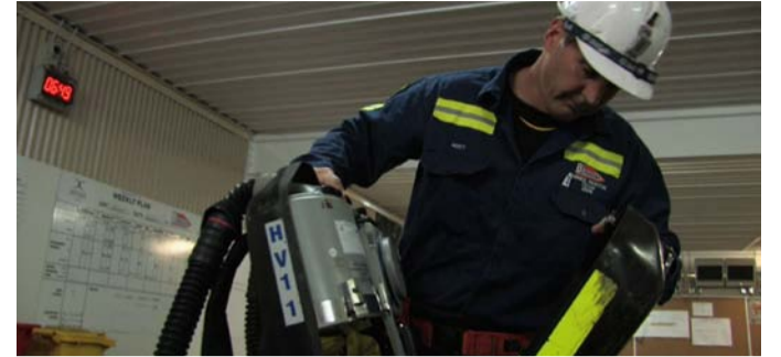
Stringent testing of the BG4 units is undertaken before and after use.
